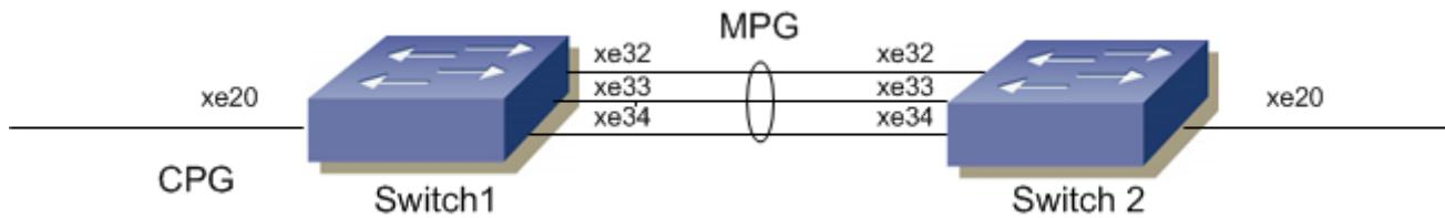
Figure 1-95: TFO with port-channel
