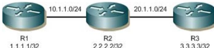
**Figure 4-111: Basic Topology of Three Routers**
