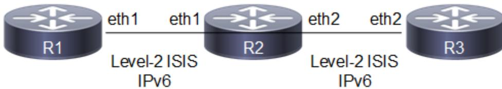
Figure 7-49: IS-ISv6 Passive Interface
