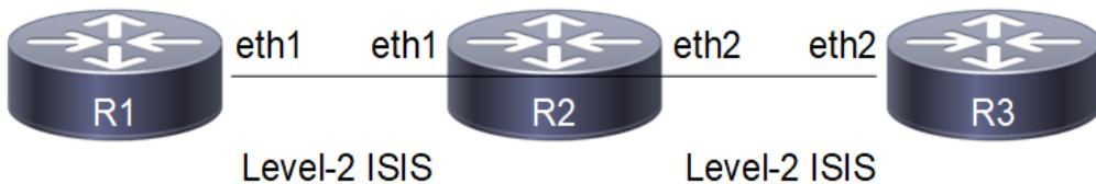
**Figure 6-40: IS-IS Passive Interface**
