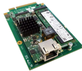
Network Module NM5 (SSD & xDSL Modem)
