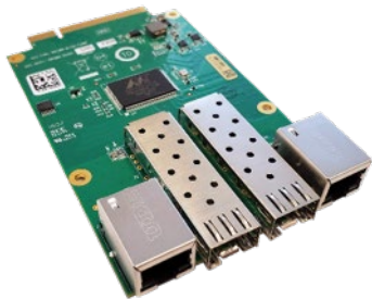
Network Module NM6 (1G auto media detect)
