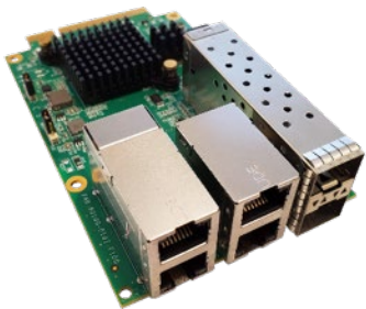
Network Module NM7 (1G RJ-45, 10G SFP+)
