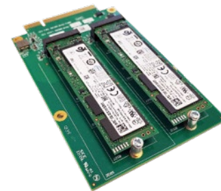
Network Module NM5 (NVMe or SATA SSDs)
