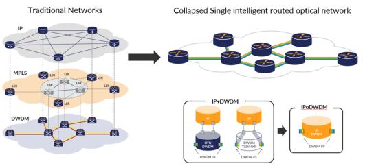
Native DWDM interfaces in the routers allow for reduction of network layers, single control plane, and network simplification.
